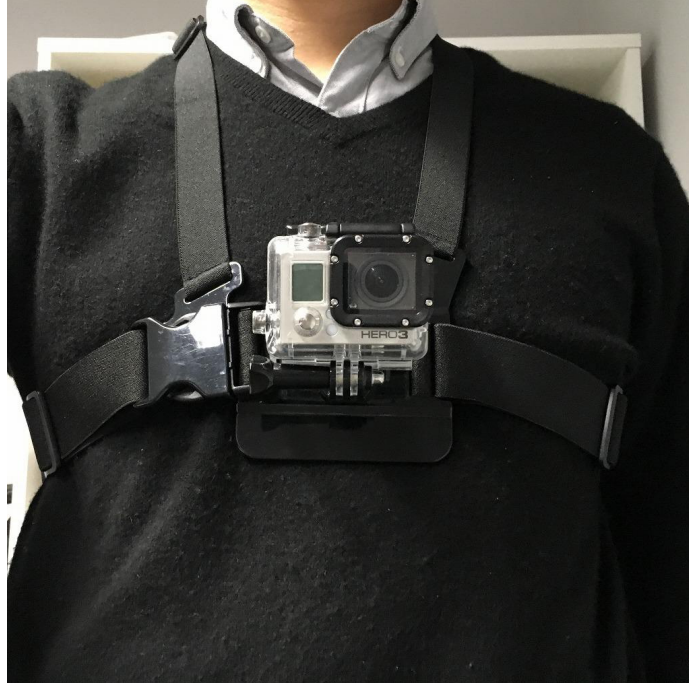
Figure 4.2.: Camera configuration: the camera is mounted on the center of the wearer’s chest.
