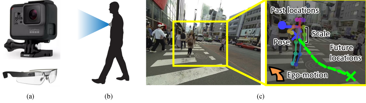
Figure 1.1.: Future person localization. (a) An example of a wearable camera (upper: GoPro HERO, lower: Google glass.) (b) Camera configuration used in this work. A wearable camera is mounted on the wearer’s chest. (c) Given a first-person video of a certain target person, our network predicts where the target person will be located in the future frames based on the poses and scales of the person as well as the ego-motions of the camera wearer.
